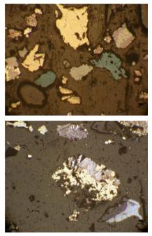
Fig. 6. Mineralogical images of polymineral Lubin concentrate (fraction > 71 □m) indicating possible and beneficial, for hydrometallurgy, galvanic interactions between minerals during leaching
