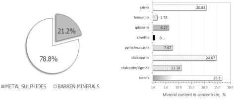
Fig. 7. Mineralogy of "high-in-recovery" Lubin concentrate used for hydrometallurgical investigations
