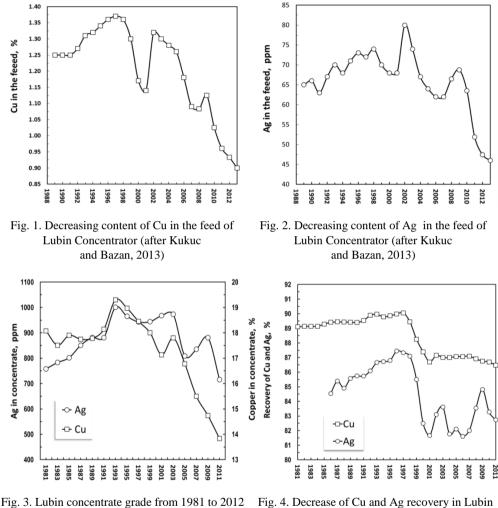
(Fig. 3) and become the main reason for growing technological concerns both in flotation and flash smelting, creating high costs of copper production.
